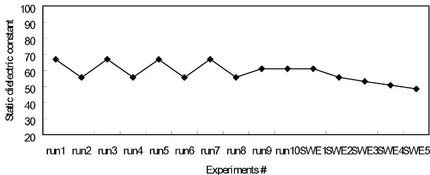
Fig. 3. Relationship between experimental conditions and static dielectric constant (Thermodynamic and Transport Properties of Water and Steam Version 1.0, 1999).
